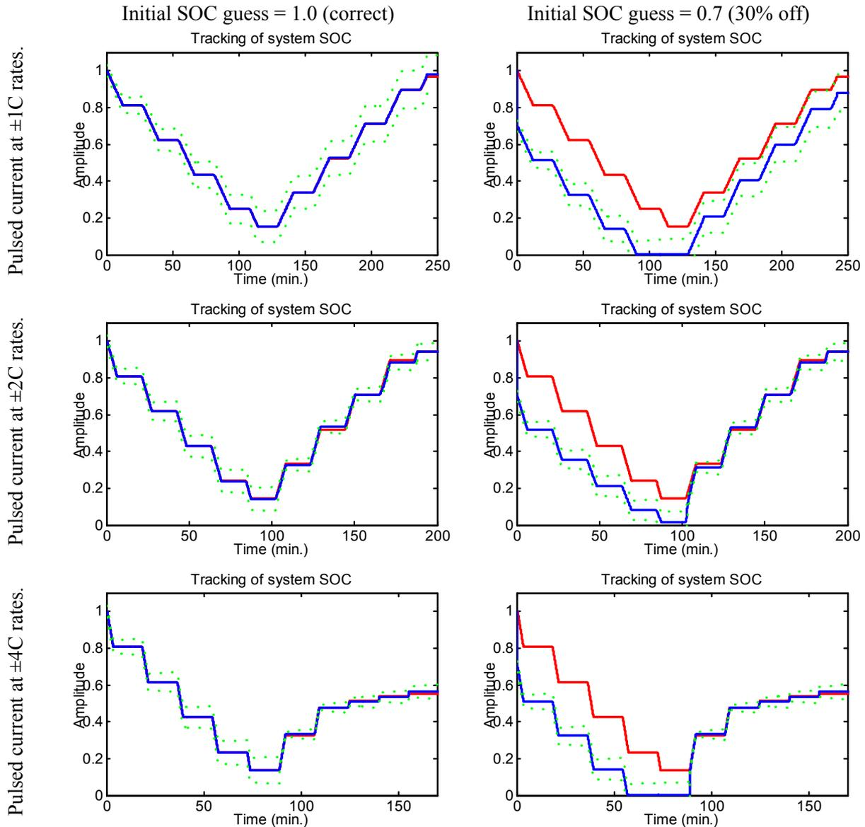
Figure 3: Filter-state tracking of SOC for correct initial estimate and incorrect initial estimate.
