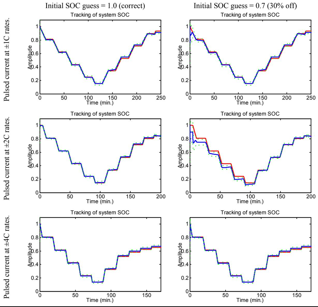
Figure 4: RBF tracking of SOC for correct initial estimate and incorrect initial estimate.
