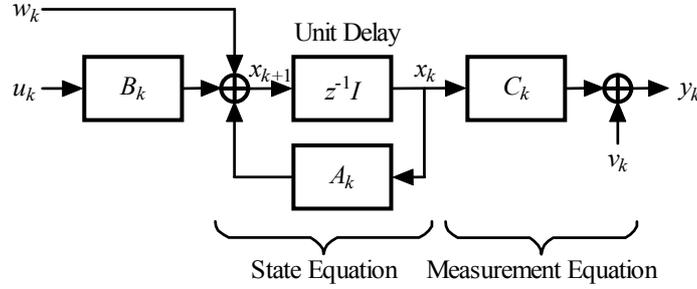
Figure 1: Diagram of system in state-variable form.
