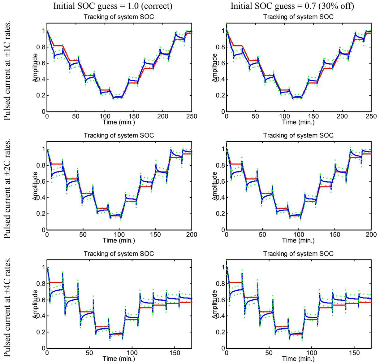
Figure 2: One-state tracking of SOC for correct initial estimate and incorrect initial estimate.
