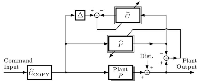
Figure 5: A system which is unbiased by disturbance.
