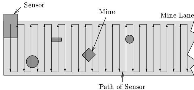
Figure 3: The movement of the sensor over the mine lane during data acquisition.
