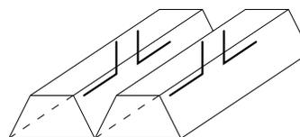
Figure 2: Diagram of the microwave horns and antennae.
