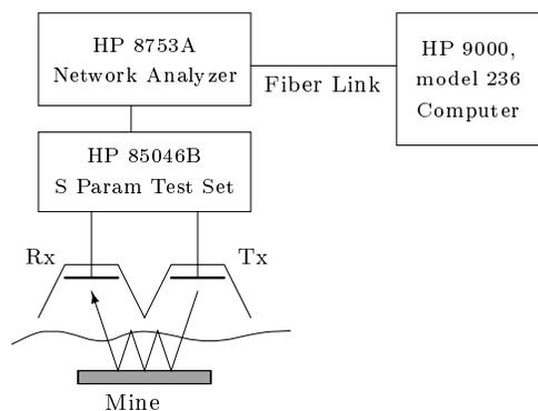
Figure 1: Block diagram of the measurement setup.
