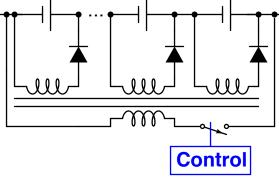
The control rapidly switches the primary; diodes route the current.
