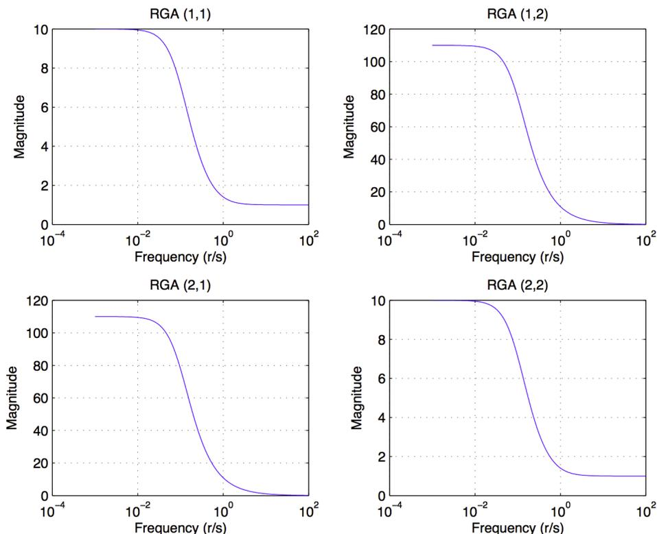
– Here we see that the RGA values are all large for the low frequency range, but off-diagonals drop to small levels for  $\omega > 1 \text{ rad/sec}$  indicating high interaction at low frequencies and  $\Lambda(G) \rightarrow I$  at high frequencies
