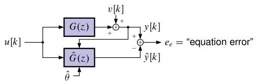
■ In the diagram, given measurements of  $\{u[k], y[k]\}, \hat{y}[k]$  is computed to be
