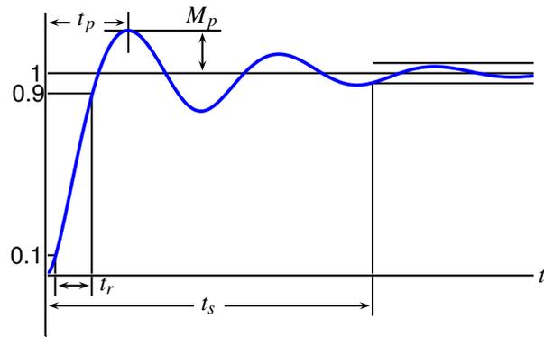
**DEFINITION:** Feedback is the process of measuring the controlled variable (*e.g.*, temperature) and using that information to influence the value of the controlled variable.
