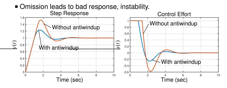
Solution = "integrator anti-windup." Turn off integration when actuator
