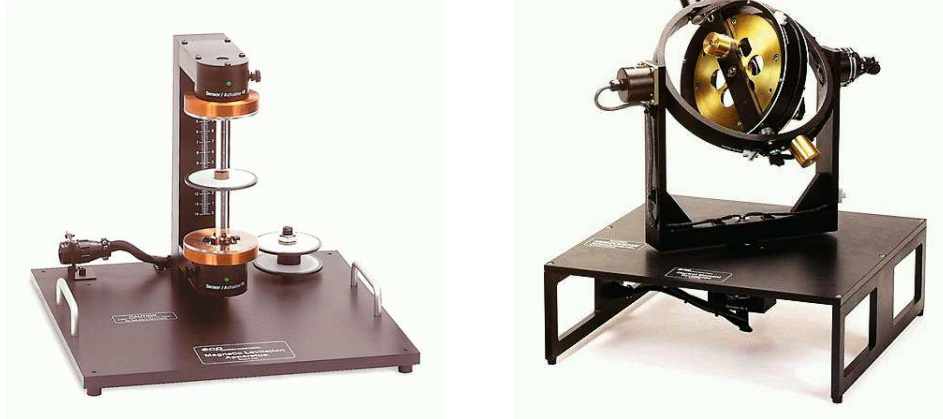
Figure 1. The two lab devices. The MagLev device is to the left; the Gyro device is to the right.
